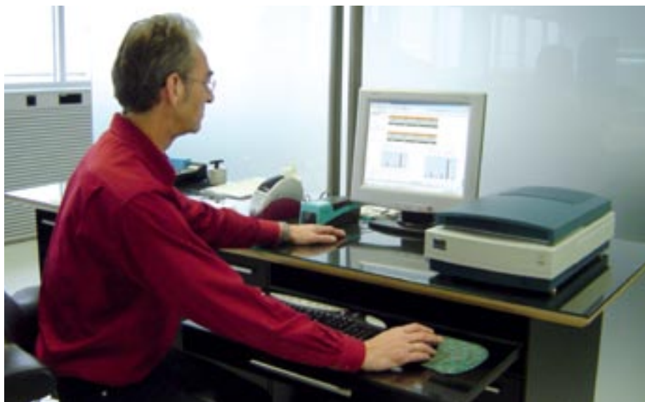
The PTS-DOMAS system converts the measurements of the Image Analyzer (on the right on the desk) into a value for evenness and a graph representing the distribution of the grey tones over the solid. If necessary, these can be compared to the values of a reference paper.
